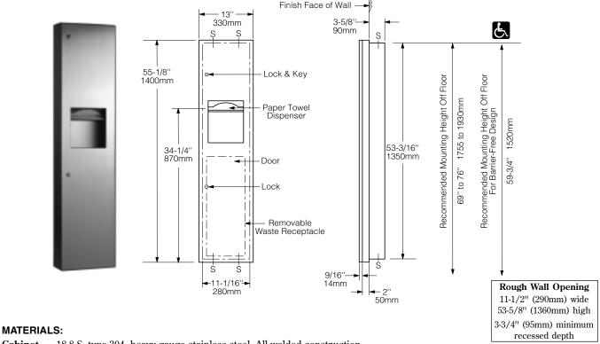
Cabinet — 18-8 S, type-304, heavy-gauge stainless steel. All-welded construction.
