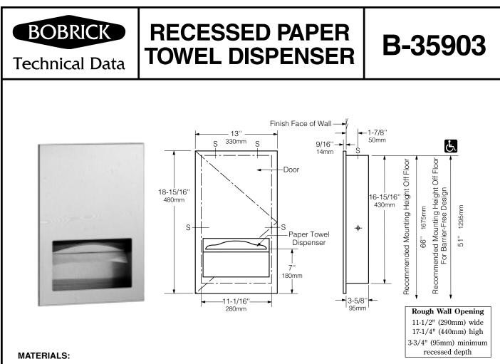
Cabinet — 18-8 S, type-304, heavy-gauge stainless steel. All-welded construction. Exposed surfaces have satin finish.
