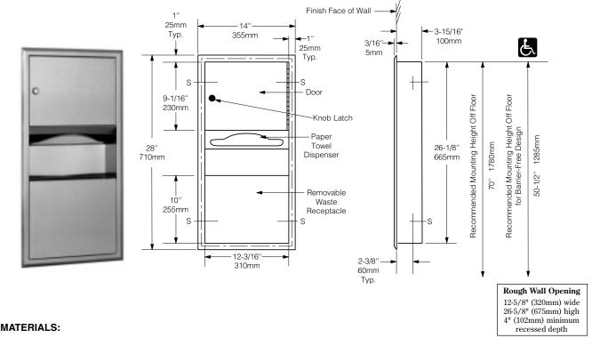
Cabinet — 18-8 S, type-304, 22-gauge (0.8mm) stainless steel. All-welded construction. Exposed surfaces have satin finish.
