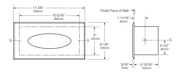
Rough Wall Opening 10-3/4" (275mm) wide 5-1/4" (135mm) high 4" (102mm) minimum recessed depth
